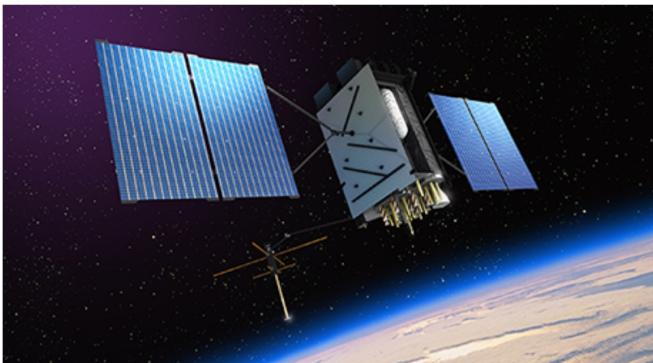
The Global Positioning System (GPS) is a space-based radio-navigation system consisting of a constellation of satellites broadcasting navigation signals and a network of ground stations and satellite control stations used for monitoring and control. Currently 31 GPS satellites orbit the Earth at an altitude of approximately 11,000 miles providing users with accurate information on position, velocity, and time anywhere in the world and in all weather conditions.
