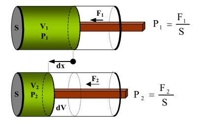
$$W_{12} = \int_{V_1}^{V_2} -P.dV$$
