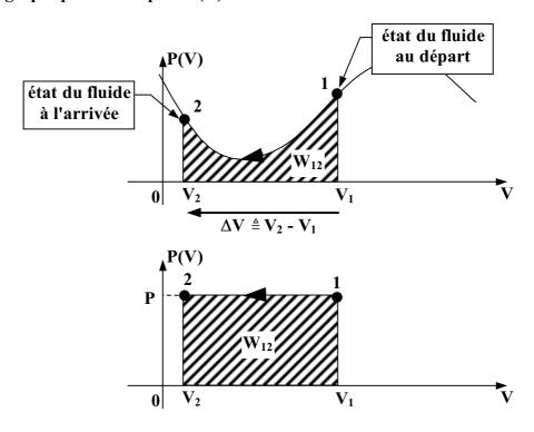
Transformation isobare  $\Rightarrow$  W<sub>12</sub> = -P  $\times$  (V<sub>2</sub> - V<sub>1</sub>)
